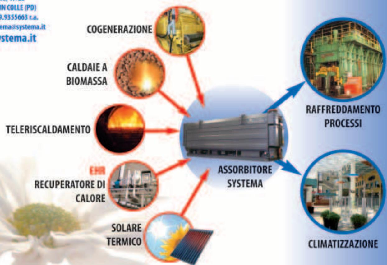
The diagram illustrates the Systema energy cycle. On the left, five heat sources are shown in circular icons with arrows pointing towards a central cylindrical unit labeled 'ASSORBITORE SYSTEMA':
